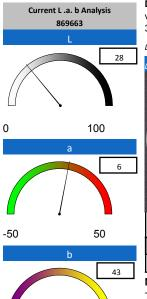
Description of Test: The process of making a patch isolates and agglomerates insoluble by-products associated with varnish. The color of the membrane patch provides a guideline as to the extent of varnish potential. Generally a value over 35 is considered abnormal.
